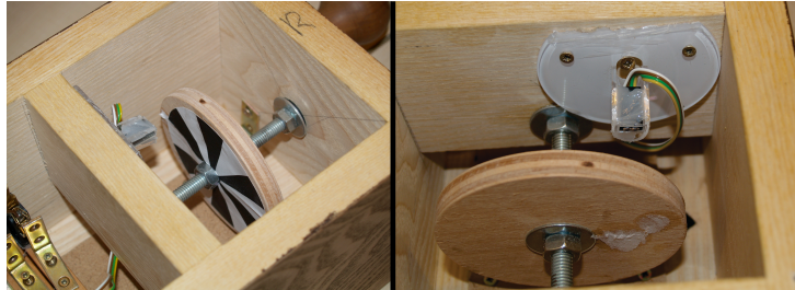
Figure 6.8: Measuring the turning of the crank using a reflection light barrier.
