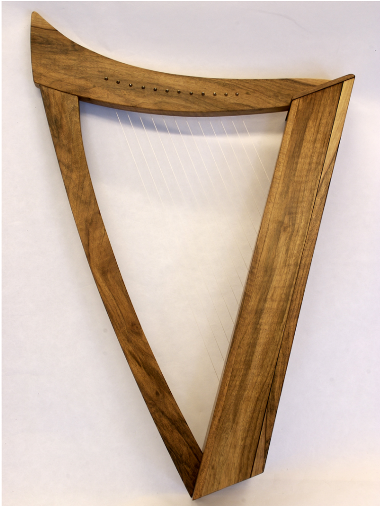
Figure 8.2: Our modified harp. The resonant body contains vibration sensors for each string and is stuffed with styrofoam to minimize acoustic sound.
