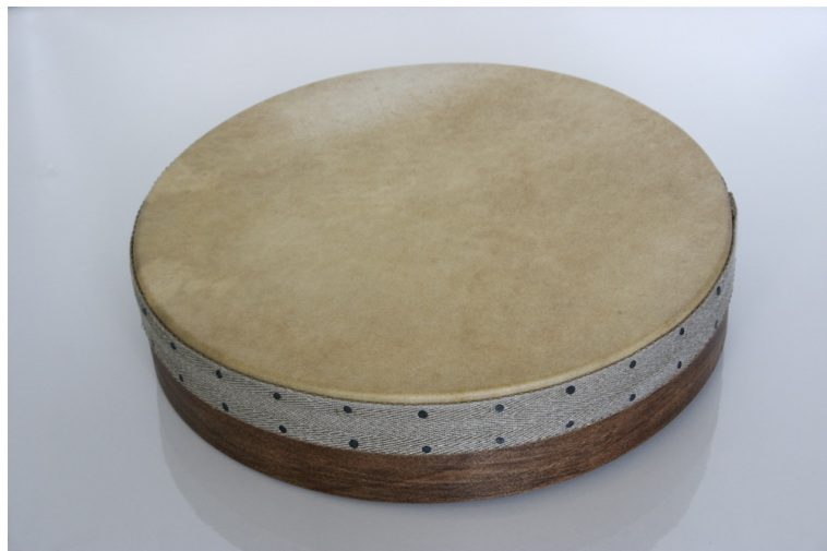
Figure 8.1: Our modified frame drum. To minimize acoustic sound, we stuffed it with styrofoam. The back is closed and has an output connector for the sensor.
