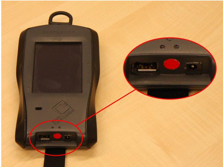
**Figure 5.1:** AIXplorer audio guide device. The magnification shows the custom FireWire audio connector and the charging socket.
