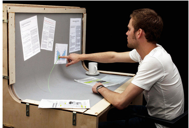
Figure 1: BendDesk seamlessly merges a horizontal and a vertical interactive surface with a curve.
