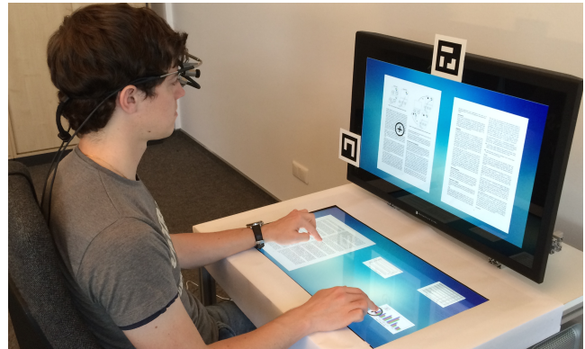
Figure 1: With help of the users gaze one can interact on the horizontal surface using direct touch and on the vertical surface via indirect touch.
