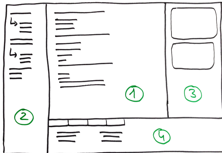
Figure 4.1: This sketch depicts basic areas of common IDEs: 1) content area, 2) project tree, 3) side panel and 4) bottom panel
