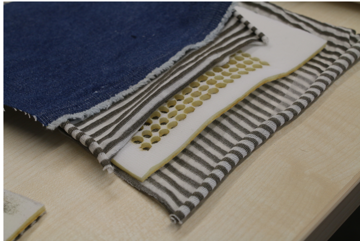
Figure 3.3: The layers of the prototype in correct order with Vliesofix already applied to the lower pinstripe fabric and jeans as potential upper layer.
