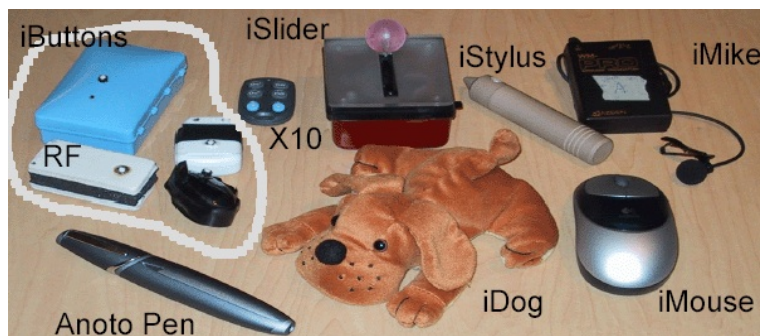
Figure 2.1: Some of the first iStuff toolkit components that can be connected wirelessly or via Bluetooth or USB.
