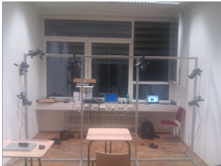
Figure 3.2: Vicon camera setup used for recording
