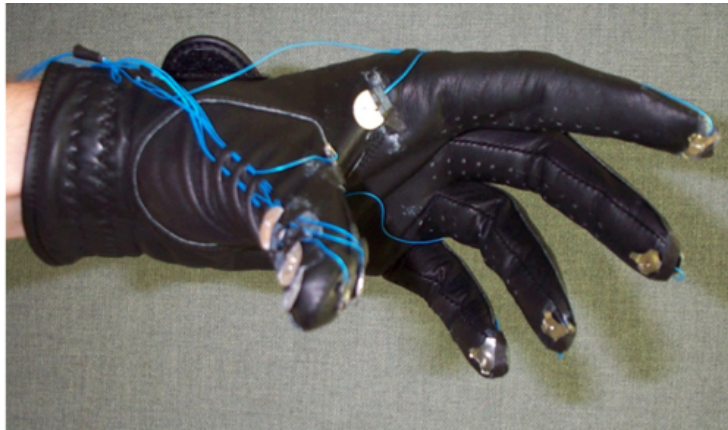
Figure 2.12: KITTY : Prototype glove system illustrating initial contact placement.
