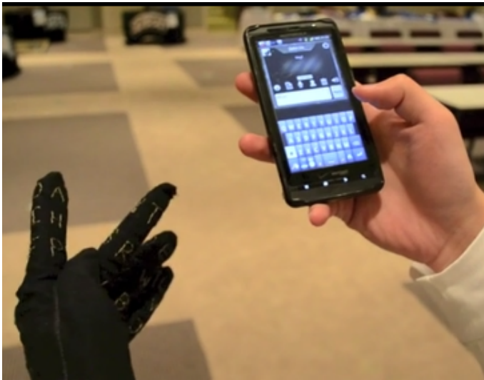
Figure 2.14: GAUNTLET : Keyboard glove implementation connected to a mobile phone via bluetooth.
