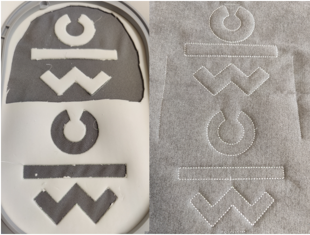
Figure 2: Creating raised and recessed sliders. First, some 3-mm foam was fixated onto an underlying thin fabric, and the slider shape was embroidered onto the foam to perforate it. Then, unnecessary foam was removed (left). Finally, surface fabric of the furniture was embroidered on top of the foam (right).
