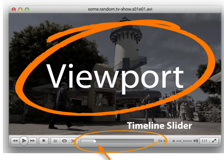
Figure 1.4: Setup of a media player, consisting of a viewport to show the content in, a timeline slider with knob (arrow), and several additional widgets for input and feedback.
