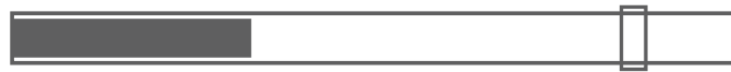
Figure 3.6: Task visualization with a progress bar. The outline shows the full range of possible values, the small rectangular outline represents the target area. The solid bar, starting from the left, visualizes the slider position. Note that the length of the outline and the dimensions of the target are dependent on the mapping specified by the condition
