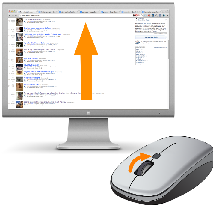
Figure 1.2: Moving the finger downwards on the mouse wheel moves the content of a website upwards.
