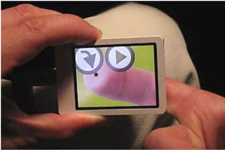
Figure 6.2: Using the back of the device to create touch input. Solves problems with occlusion from the fingers. Taken from Baudisch and Chu [2009].
