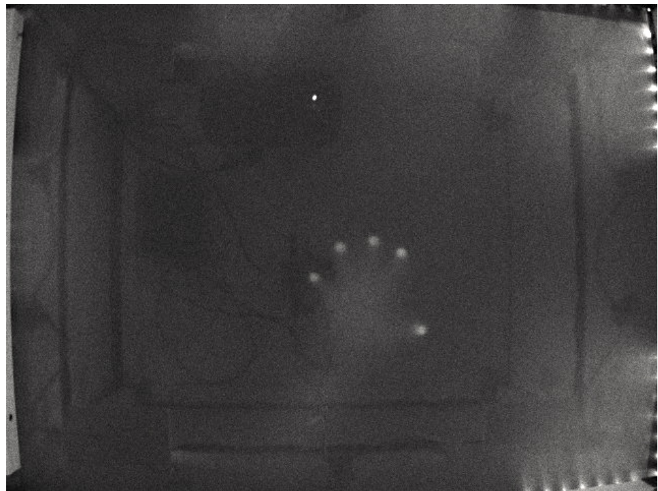
Figure 2.8: The view from the camera beneath our multi-touch tables. This image is background subtracted, thresholded, and then processed using a connected component analysis. This gives us the five bright spots—the fingers touching the surface.
