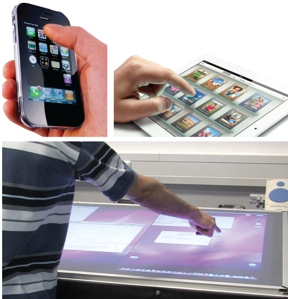
Figure 1.2: Different form factors of touch-capable devices. The larger the device, the more body parts are involved in the interaction and the less precise is the interaction with the device.
