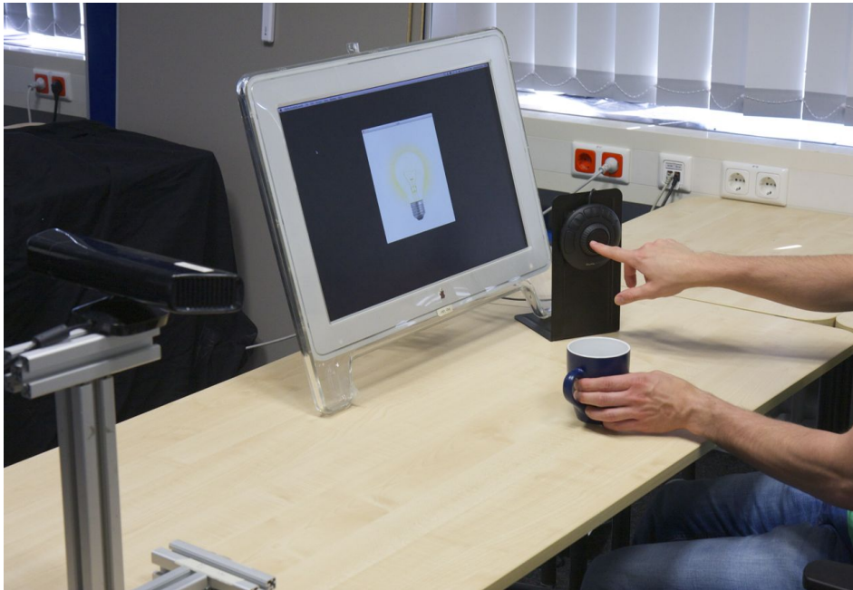
Figure 7.6: Setup of the system for the light scenario (left to right): Kinect, display, mug, rotary knob. The user is programming the mug by demonstration: mug and rotary knob used to control the light are rotated at the same time. From now on, the user can rotate the mug to dim the light visualized on the screen. Taken from Corsten et al. [2013].
