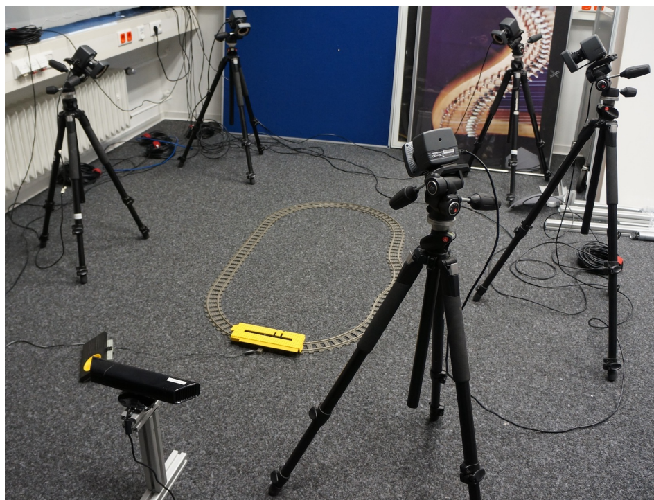
Figure 5.4: Our test setup with the toy train tracks and the VICON cameras. Image adapted from Avellino [2013].
