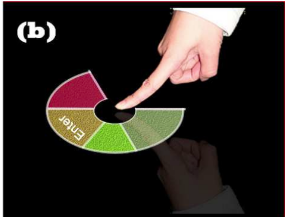
Figure 1.5: Finger orientation selects entries from a pie menu. Taken from Wang and Ren [2009].
