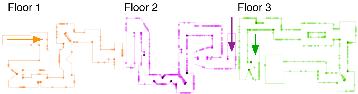
Figure 10: Collisions for each level across all methods. They primarily occurred at bottlenecks and in corners.
