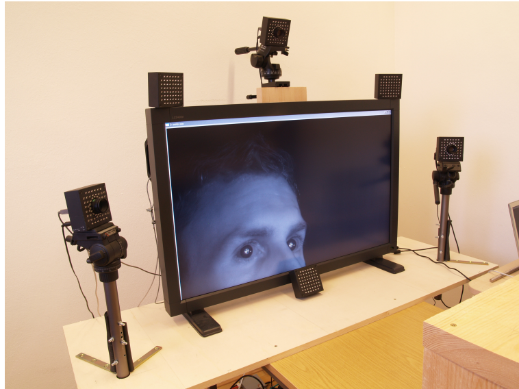
Figure 4.1: The hardware setup consisting of three cameras and three additional off-axis LEDs
