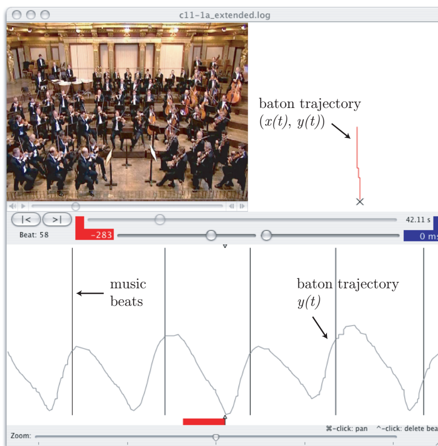
Figure 3.4: Screenshot of the BeatVisualizer program, which we wrote for visualizing users' baton gestures and marking their beats. The data shown is from a conductor.
