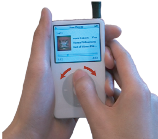
Figure 6.9: Navigating an audio timeline using the iPod click wheel. Clockwise gestures advance the audio position forwards, and counter-clockwise gestures backwards. No audio feedback is given whilst scrolling on a standard iPod.
