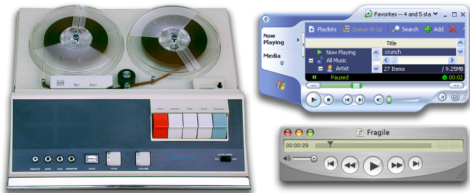
Figure 1.1: A comparison of a 1966 RCA YHS-18J tape recorder and current versions of Windows Media Player and QuickTime Player. The fundamental interaction metaphors have not changed, and modern media players continue to use the decades-old “play”, “pause”, “fast-forward” and “rewind” controls as the primary means for controlling media playback.
