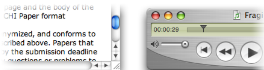
Figure 7.1: The scrollbar for document navigation (left) is analogous to the timeline slider for audio navigation (right). The wiper inside the scrollbar, which controls the current viewing area in a document, is the playhead in an audio timeline slider. The arrow buttons at either ends of a scrollbar correspond to the fast forward and rewind buttons.
