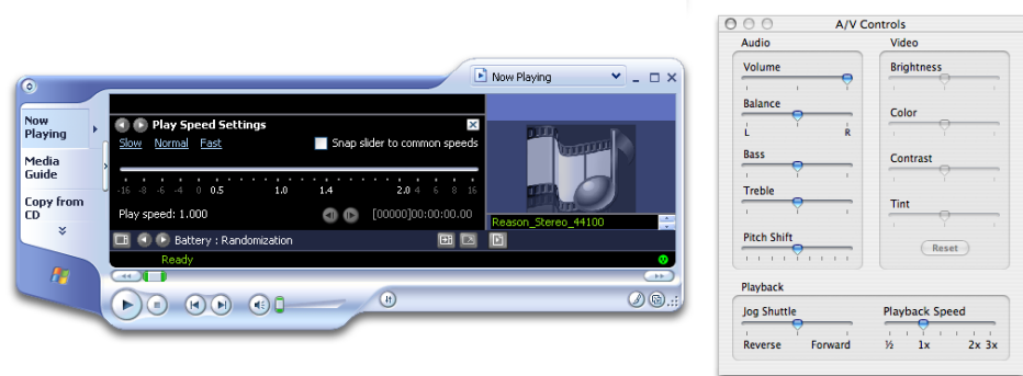
Figure 1.2: Recent versions of Windows Media Player and QuickTime Player allow media playback at rates other than one. However, the range of allowed rates is limited, and this control is offered as an advanced setting in the interface.
