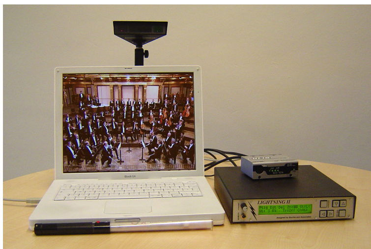
Figure 3.3: Devices used in our conducting experiment: 14" iBook laptop computer and a Buchla Lightning II baton and tracker.
