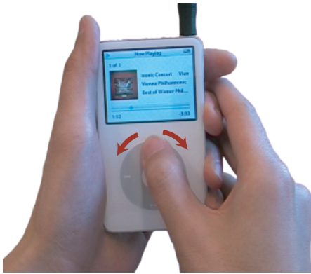
Figure 2: Navigating an audio timeline using the iPod scroll wheel. Clockwise gestures advance the audio position forwards, and counter-clockwise gestures backwards. No audio feedback is given whilst scrolling on a standard iPod.
