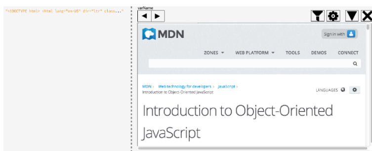
Figure 6.9: We proposed a three-column design, in which the right column can be used for detailed visualizations of runtime data. In this screenshot, the leftmost column that contains the source code is not shown. The central column shows one line of runtime information for an HTTP GET request that returns the complete HTML source code of a website. A user configured a widget to be displayed in the third column that renders a realistic preview of the HTML code. Figure Source: [Wolf, 2014]
