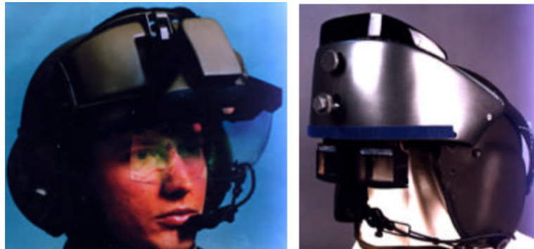
Figure 2.1: Head-Mounted Displays (HMD) have already been used in early Augmented Reality research [Azuma, 1997].
