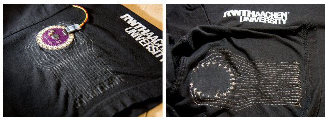
Figure 3. Lines of conductive thread sewn into the sleeve of a T-shirt and connected to a microcontroller board (left: outside, right: inside). Lines are spaced approx. 2mm apart. On the outside, the lines are also painted on for demonstration purposes—normally the black outer cotton thread would be invisible.
