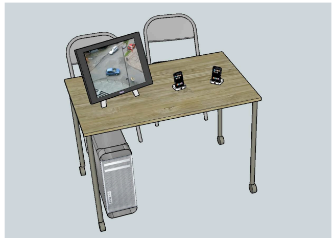
Figure 3: Sketch of the PocketDRAGON demonstrator setup. The two mobile devices are running PocketDRAGON, the stationary computer is the trajectory server which can also show the desktop version of DRAGON for comparison with PocketDRAGON.
