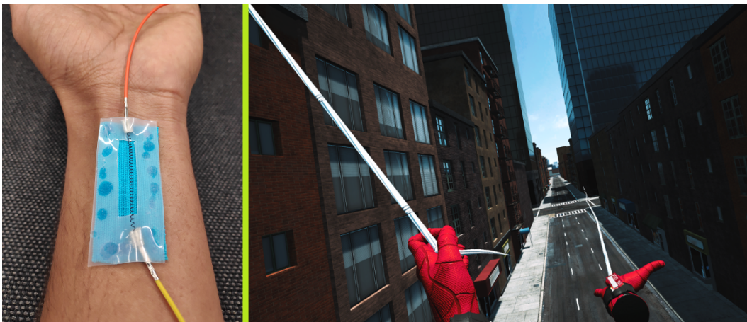
Figure 3.5: Left : Pincher on the wrist to create a haptic web-shoot illusion. Right: Visual web-shoot experience in the Spiderman game - Image credit: http://createvr.com/spider-man-far-from-home (accessed: 17.11.2019)
