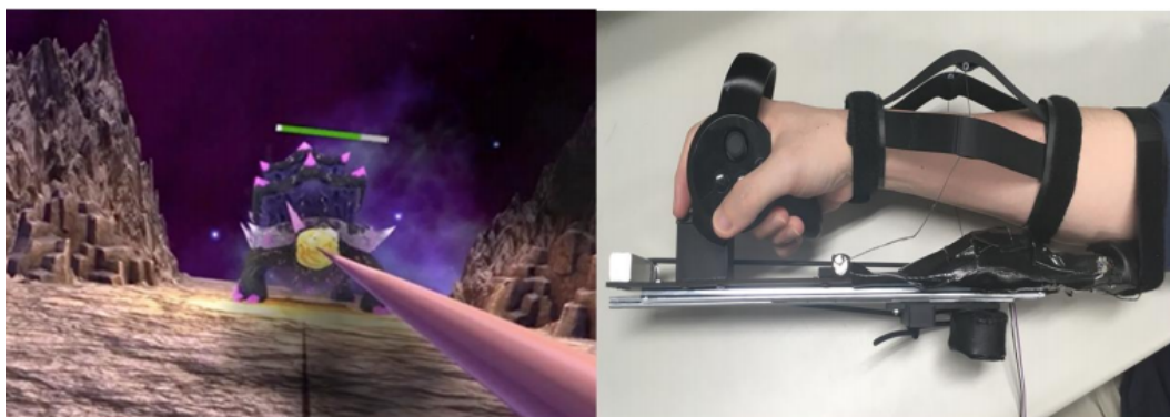
Figure 2.5: Skin stretch to deliver superficial hand extension in Virtual Reality games [Yamashita et al., 2018]
