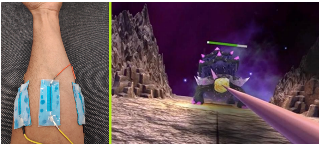
Figure 3.4: Left : Pinchers positioned parallelly on the arm to create long-arm illusion in VR games. Right: Visual arm-stretch experience in a VR game [Yamashita et al., 2018]
