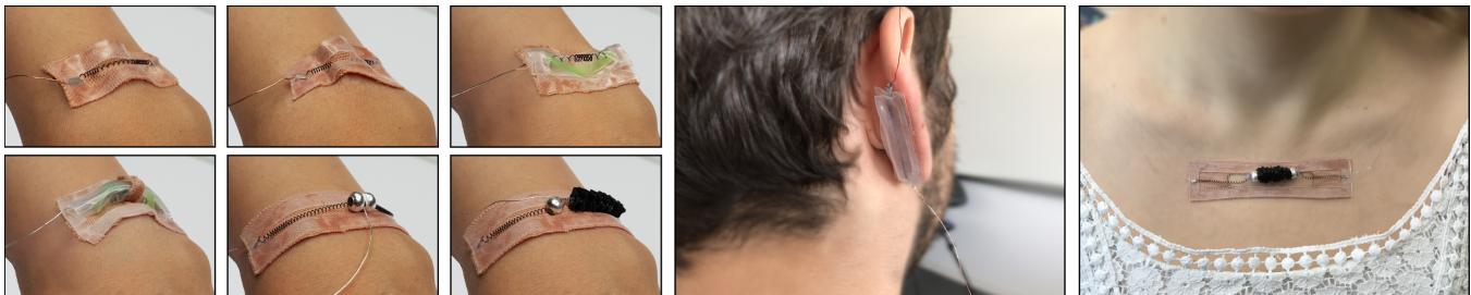
Figure 1: Springlets on-skin stickers enable expressive mechanotactile output on the user's skin. They use shape memory alloy springs to achieve a thin, flexible, and silent form factor that can be worn on challenging body locations and near the head.
