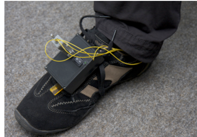
Figure 2. One of our sensor boxes attached to a shoe. The box is held in place by a flexible ruler that is secured underneath the shoelaces.
