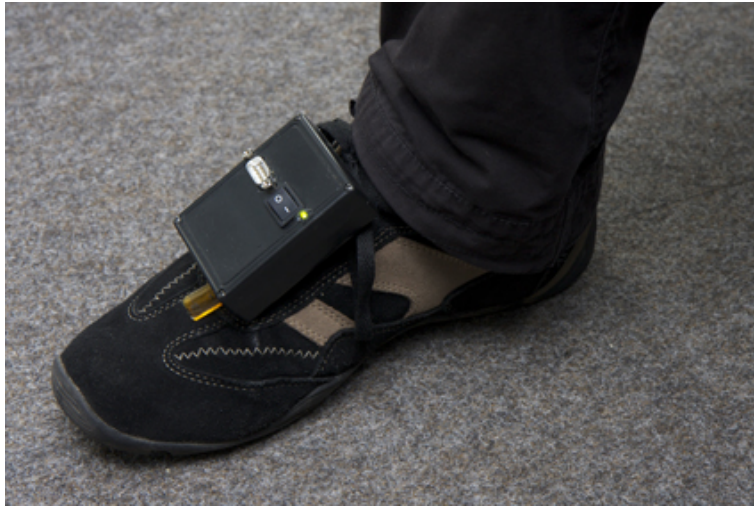
Figure 4.2: One of our sensor boxes mounted on a shoe
