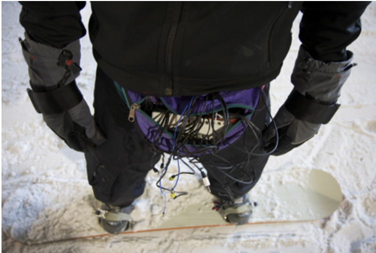
Figure 4.1: Wires and belt bag of the snowboard training system.
