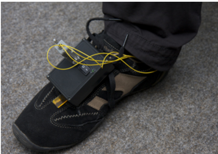
Figure B.6: A sensor box with attached sensor cables.
