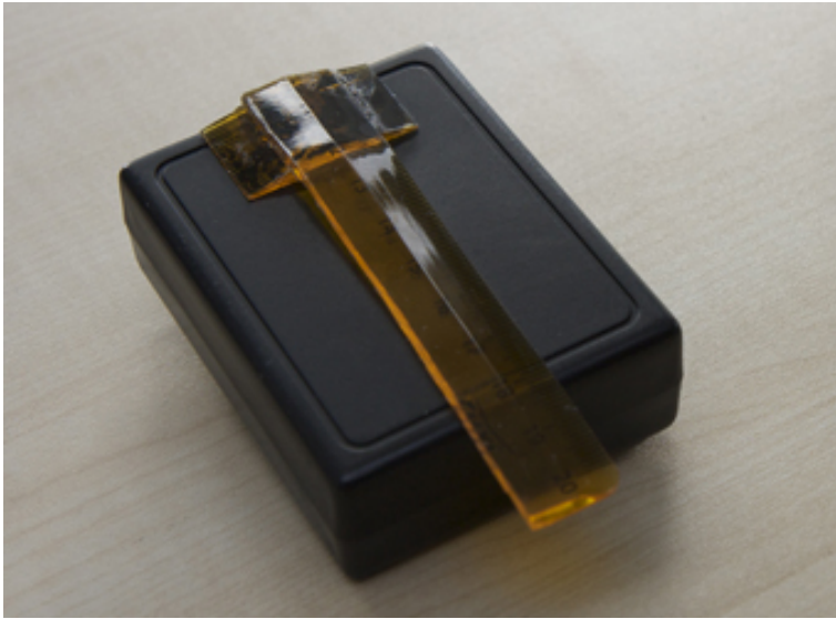
Figure B.5: The bottom of one of Saltate!'s sensor boxes. The ruler is flexible and can be pushed under a shoe lace.
