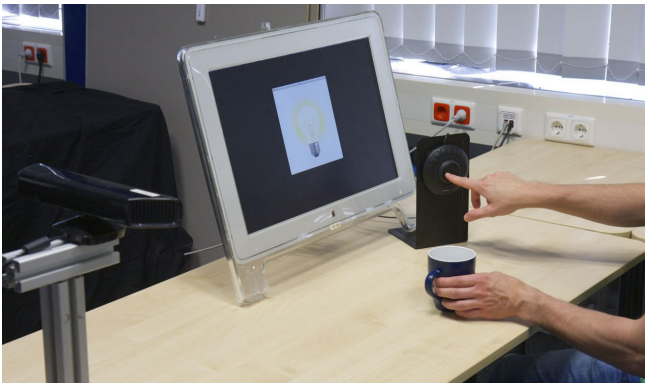
Figure 7. Setup of the system for the light scenario (left to right): Kinect, display, mug, rotary knob. The user is programming the mug by demonstration: mug and rotary knob used to control the light (on screen) are rotated at the same time. From now on, mug rotation dims the light.
