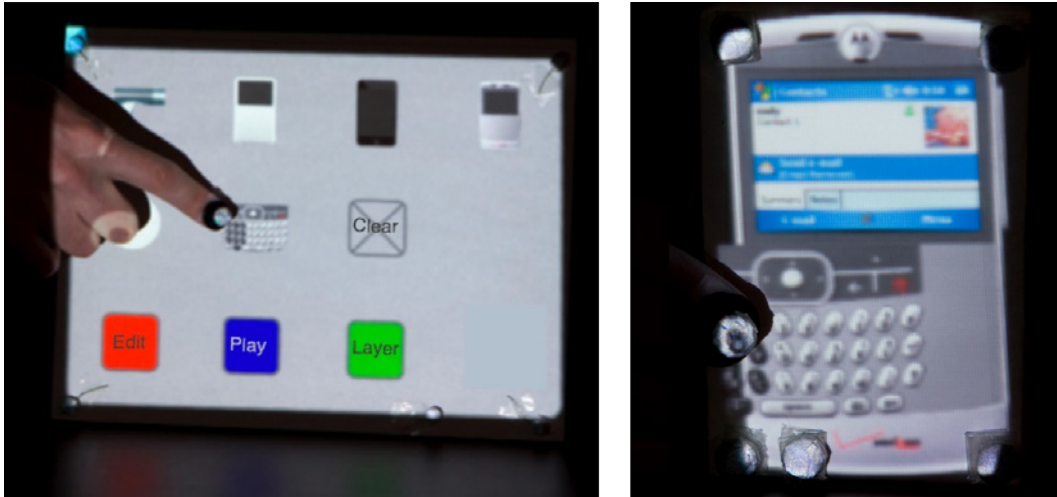
Figure 2.9: Palette with interaction styles (left) and physical mockup with a virtual interface (right). The user touches an UI widget on the palette and drags it to the naked prototype for adding the widget to it.
