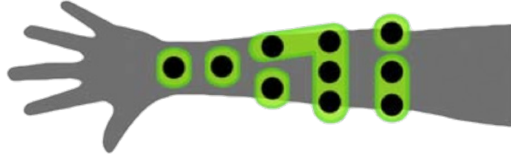
Figure 2.4: Input accuracy achieved by Skinput. Worn above the elbow, the sensor can distinguish six touch zones on the user's forearm featuring a touch detection of true positives by 88,8%.
