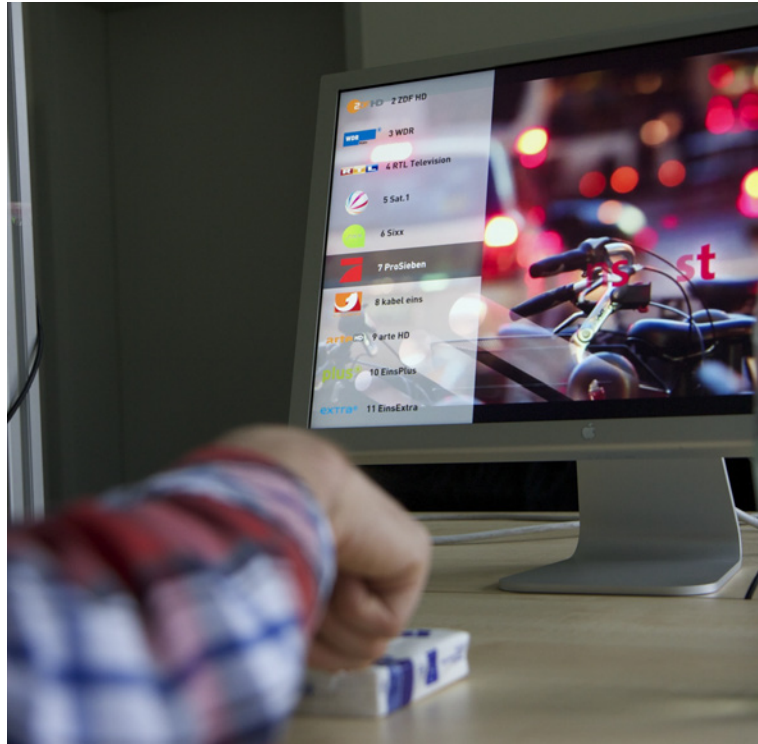
Figure 5.17: Tissues in action. A user is pushing the lower third of the pack of tissues with his forefinger for navigating the channel list one step down.
