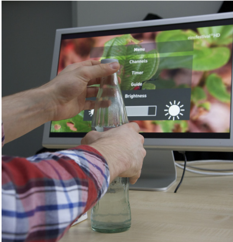
Figure 5.18: Bottle in action. Similar to volume control, brightness was controlled by turning the bottle or its cap. However, prior to that, brightness mode had to be activated via the menu by using the tissues.
