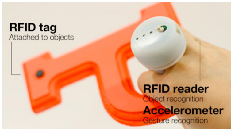
Figure 2.7: End user programming with OnObject. The user puts an RFID tag to the object (“P”) to be programmed and executes an acceleration-based gesture while holding the reader. It reads the tag, captures the gesture, and records the user’s voice.
