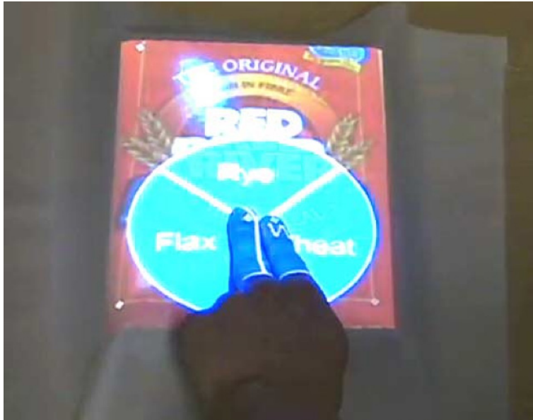
Figure 2.6: The Cloth Displays prototype. As soon as the piece of cloth drapes an object, it adopts the artifact shape and provides a touch-sensitive GUI.
