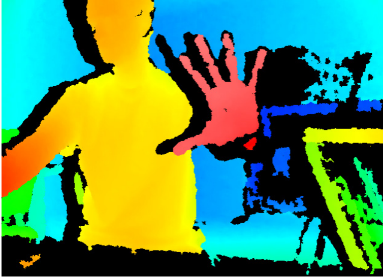
Figure 5.3: Colored depth map. This picture has been taken by a depth camera (Kinect). Reddish parts appear closest to the camera, whereas greenish parts are farthest away.
