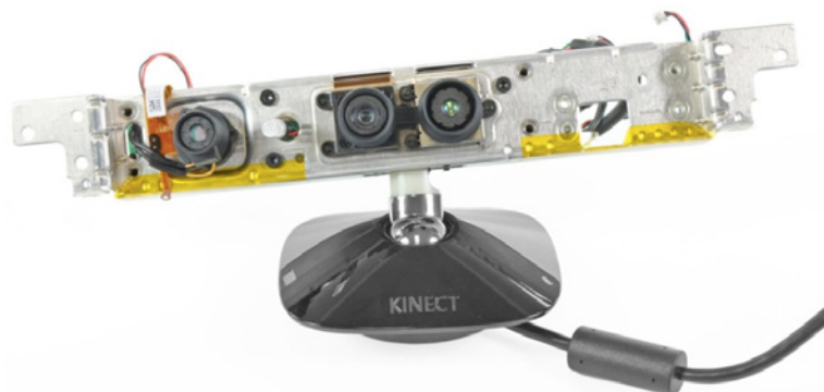
Figure 5.2: Kinect teardown. Basically, the Kinect consists of three components (from left to right): an IR projector, an RGB camera, and an IR camera. (Image: iFixit.com)
