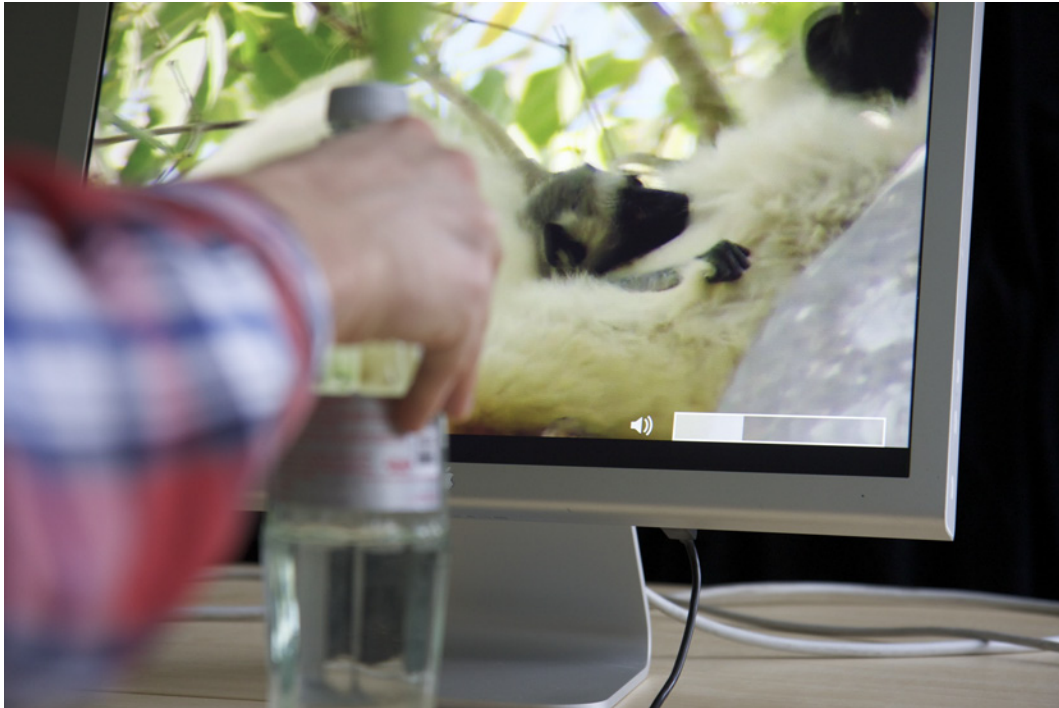
Figure 5.16: Bottle in action. A user is turning the bottle clockwise in order to increase the volume of the TV. Visual feedback is given via the volume level indicator.
