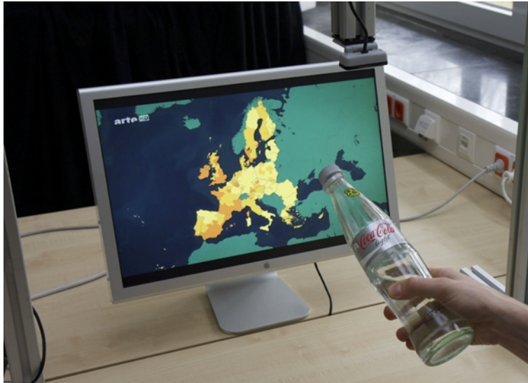
Figure 5.6: Object activation via pointing. The user points the bottle at the TV. Meanwhile, the small web camera (top) captures the green marker attached to the bottle. After three seconds of pointing, the bottle is activated.
