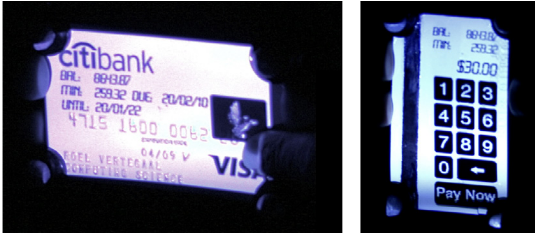
Figure 2.10: An augmented credit card (left: front side, right: back side). Display-Objects has been used to add a graphical user interface (back side) for being able to transfer payments directly.
