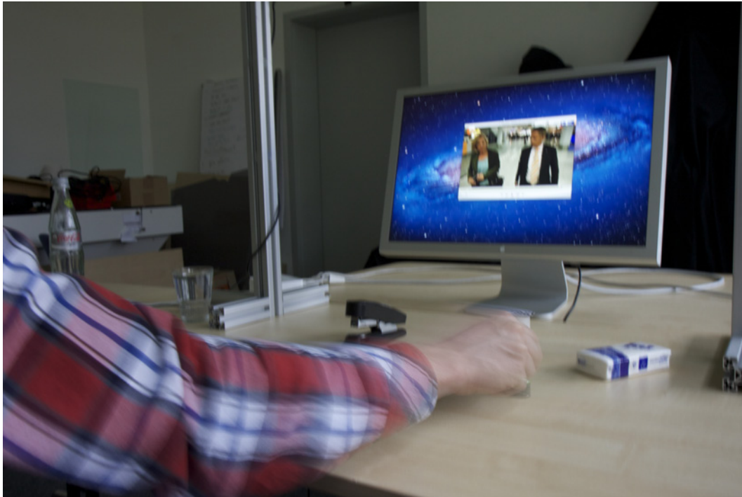
Figure 5.15: Glue stick in action. A user is sliding the glue stick to the right for dragging the timeline slider to the same direction in order to forward the video.
