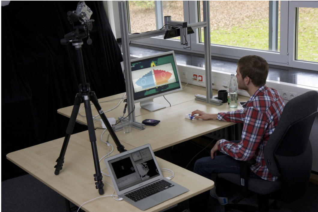
Figure 5.12: Study setup. The user (sitting on the chair) was meant to manipulate objects on the table beneath the aluminum mounting. The monitor behind the mounting served as display for the scenario applications. Object manipulation was captured by camera (fixed on a tripod). The principal investigator sat behind the laptop which served as control panel.
