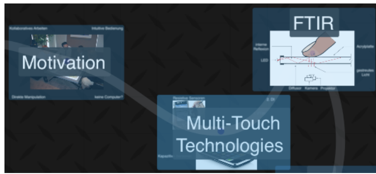
Figure 5.3: Stop layers. Each of the three blue shapes covers the dimension of a stop. A click on a layer zooms the stop in and forwards the video (basic stop-based navigation).
