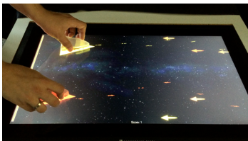
Figure 4: A space-invader game in which PERC tangibles are used as space ships.
