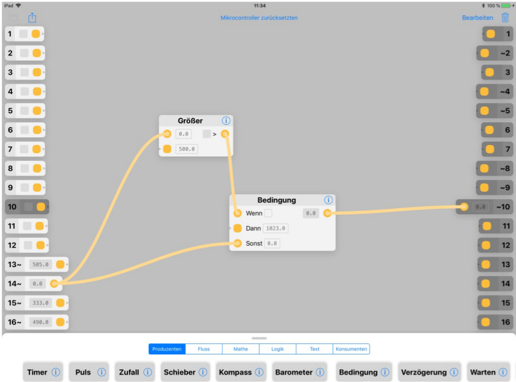
Fig. 6. Flowboard’s editor for the programming task: make an LED shine weakly resp. brightly, depending on whether a force sensor exceeds a threshold. In comparison to figure 4, pin 10 is greyed out as input pin on the left as it is used as an output pin on the right [11].
