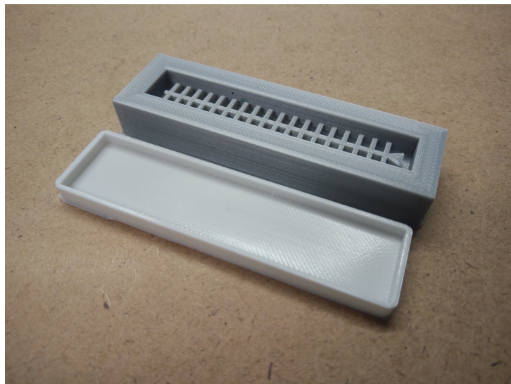
Figure 5.6: 3D-printed molds for the main body and the base layer.
