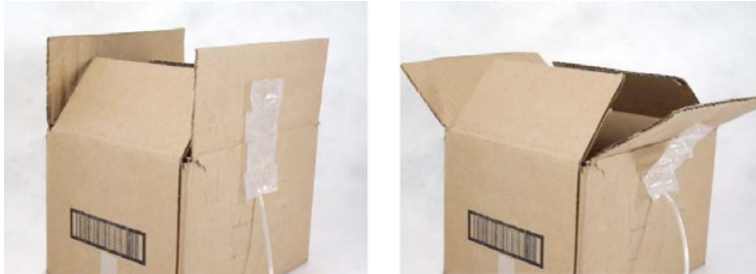
Figure 3.2: “Sticky actuators” are used to open and close a box. Niiyama et al. [2015].
