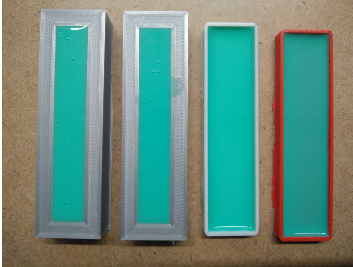
Figure 5.8: Molds filled with silicone rubber.
