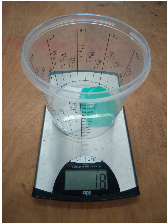
Figure 5.7: Mixing the catalyst and the basis of the silicone rubber
