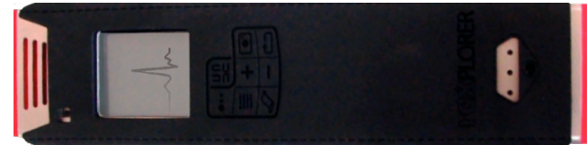
figure 2. The REXplorer measurement device consists of a Nokia N70 mobile phone and a GPS receiver packaged together in a protective shell. A soft overlay transforms the standard phone keypad to an 8 key game interface.
