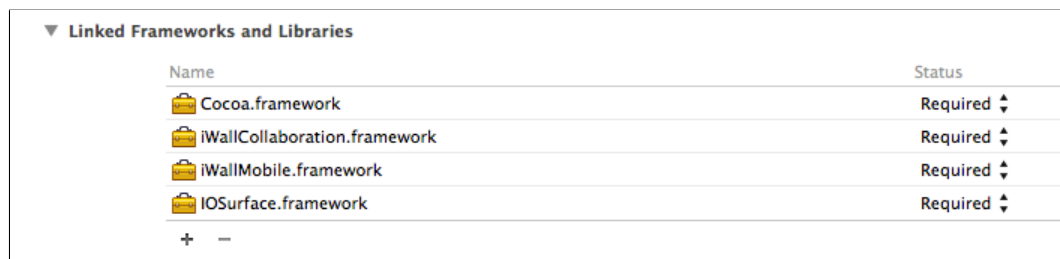
Figure A.1: Screenshot after adding iWallCollaboration.framework , IOSurface.framework and iWallMobile.framework to the Xcode Project.
