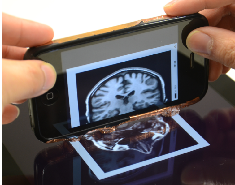
Figure 2.1: iPhone as tangible can display information on third axis as shown by Li and Kobbelt [2015]
